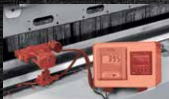
Checking subnozzle efficiency
